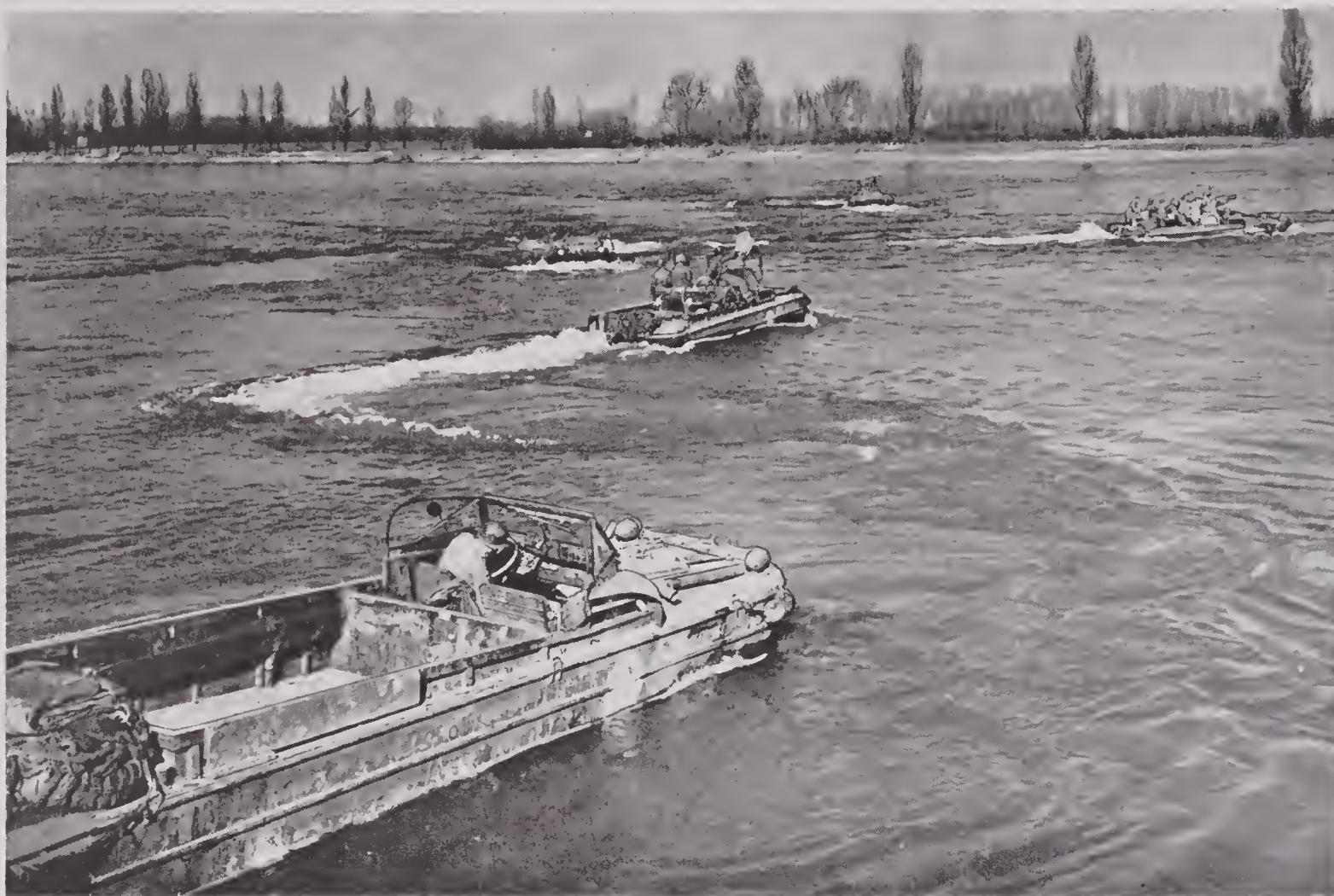
FIGURE 30. DUKWs must point well upstream when crossing swift current in Rhine River.
